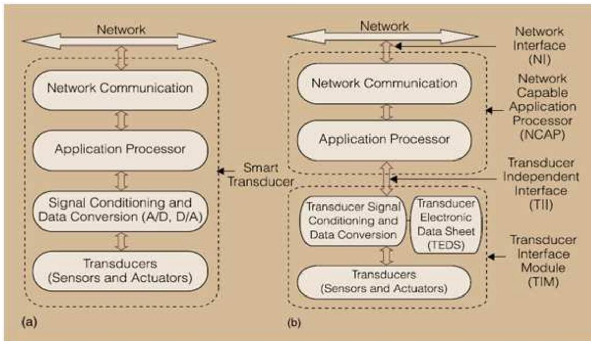
**Figure 3: (a) Smart Transducer Model (b) This Architecture Adds TEDS and the System Partition into NCAP and TIM, with a TII**
